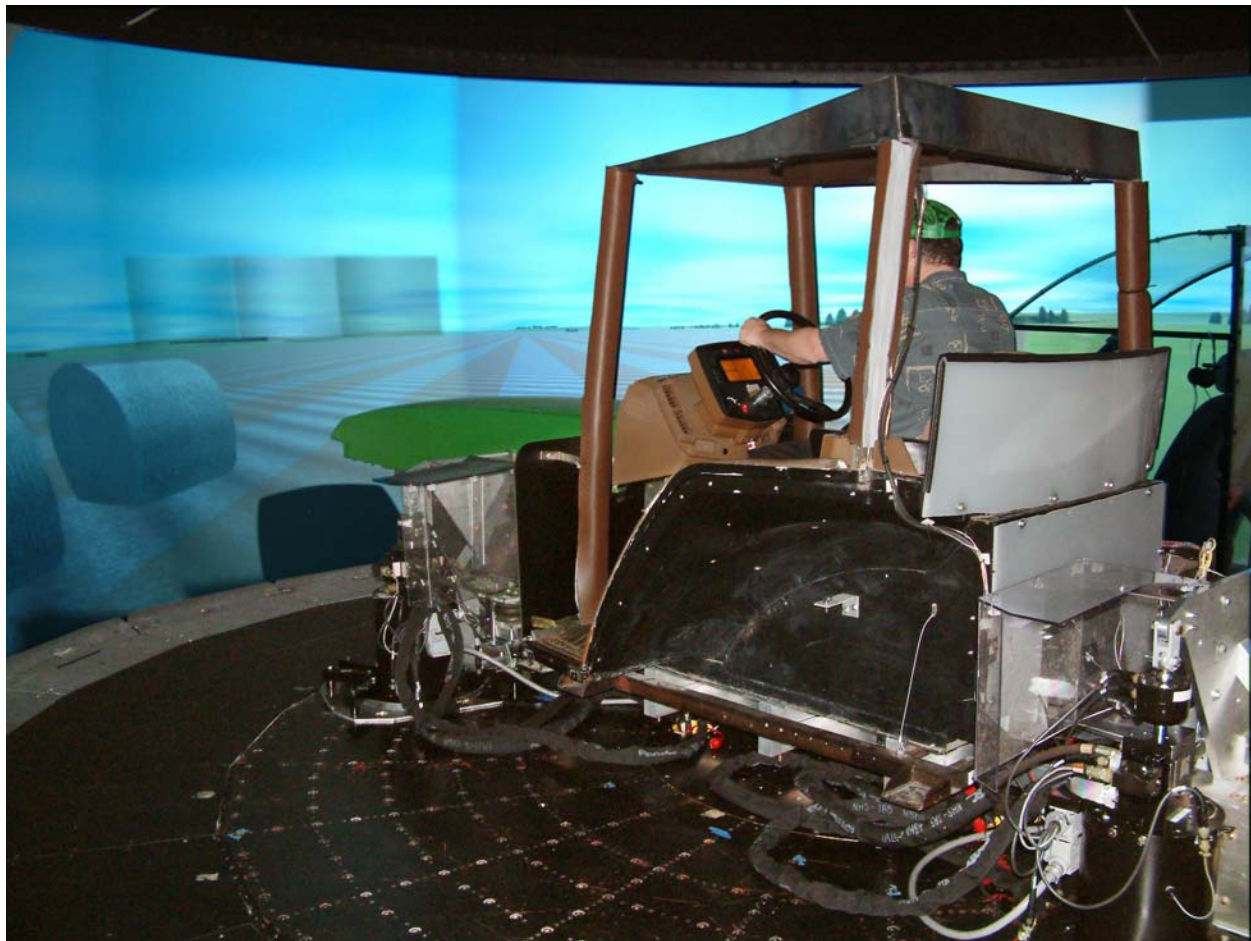
FIGURE 3 Tractor Cab in NADS Dome.
